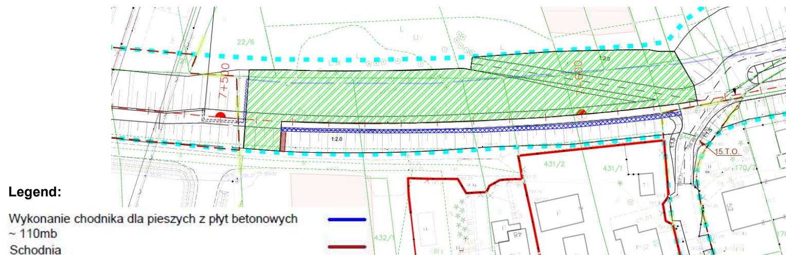
STAGE 1 - Crossing between Bugaj Street and Pod Wierzbami Street during works on the embankment's upstream side (from the side of the Vistula River).
